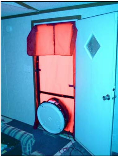
Figure 4-9. Blower door test.
